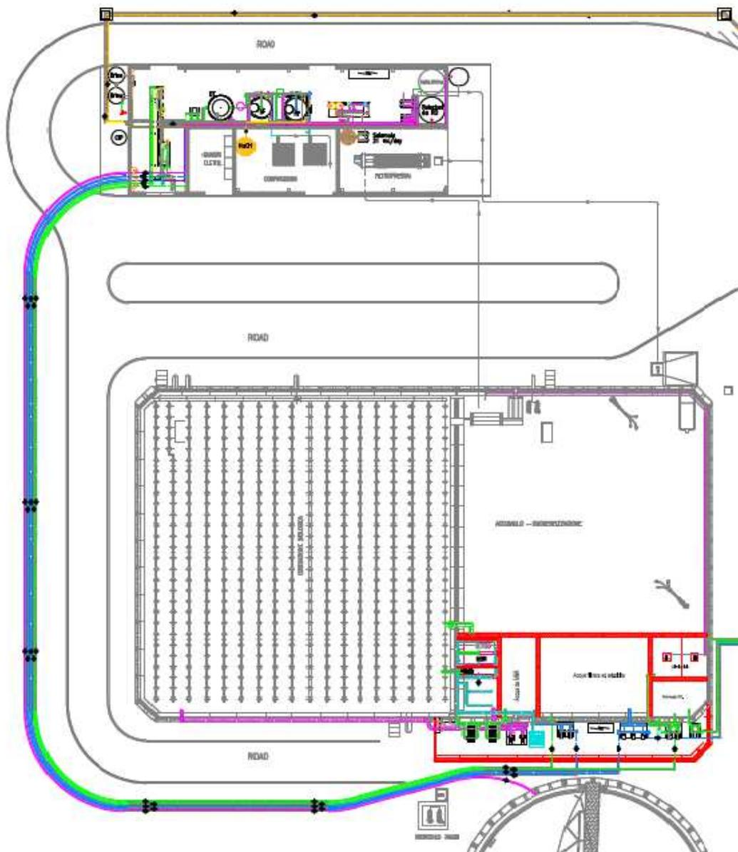
**Figure 1: Plant's layout: new civil works in red; new machineries and equipment in different colors; existing plant in gray**
