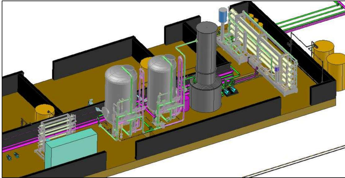
**Figure 2: 3D view of filters, RO and NF systems**
